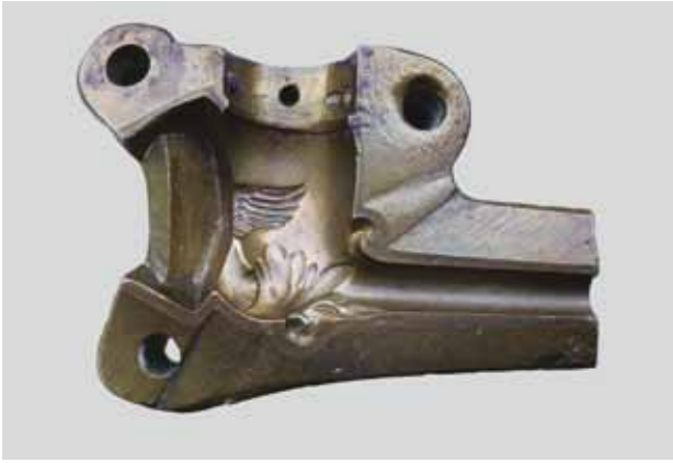
Figure 32: Part of a pipe mould, model: Crème Cupidon, no. 1290. Collection author.
